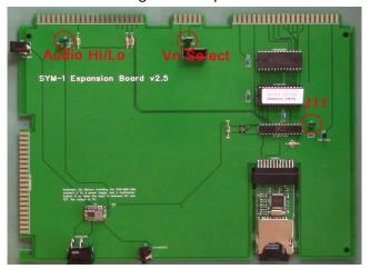
RAM on the SYM-1, a jumper should be installed at J11. If there is 0K RAM in the SYM-1, the jumper should be removed from J11 (leaving only the bare pins).
